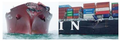
Photos sent to TradeWinds show Al Gharrafa appears to have suffered serious bow damage while the Hanjin Italy appears to show dents and scrapes to its hull and a split container amidships on its starboard side.
